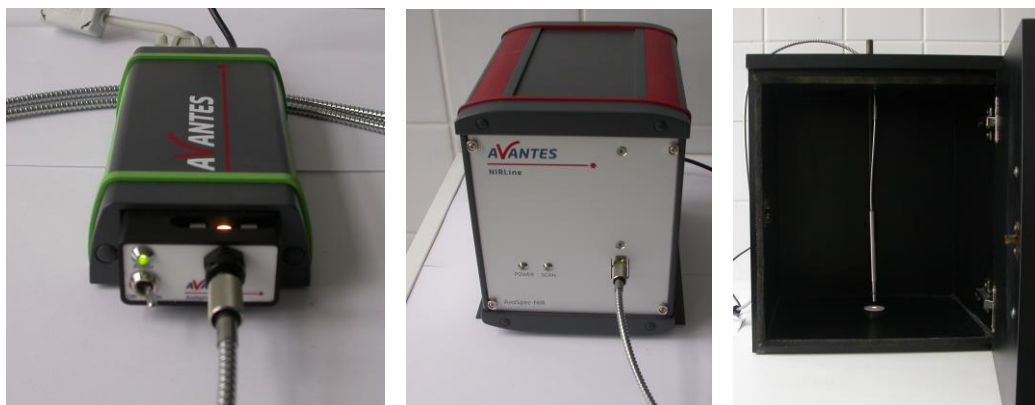
Figure 2. Light source, detector and sampling black box of the applied spectrometer
